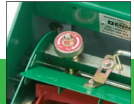
Easy adjustment of bottom blade to cylinder
