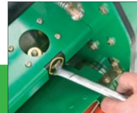
Adjustment of cylinder to bottom blade easy and positive with a single spanner
