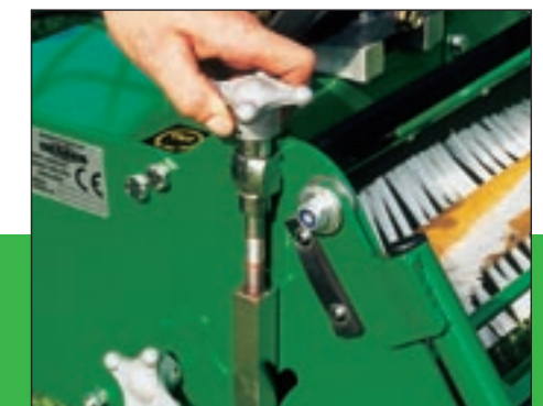
Simple single point adjustment for height of operation
