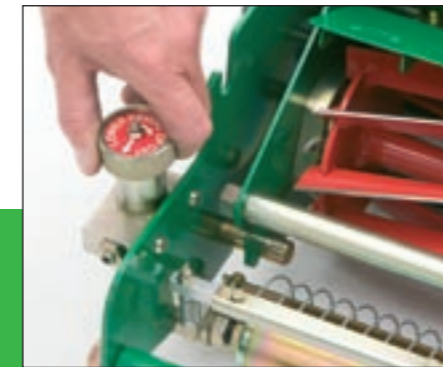
Positive, easy height of cut adjustment in 0.5mm increments
